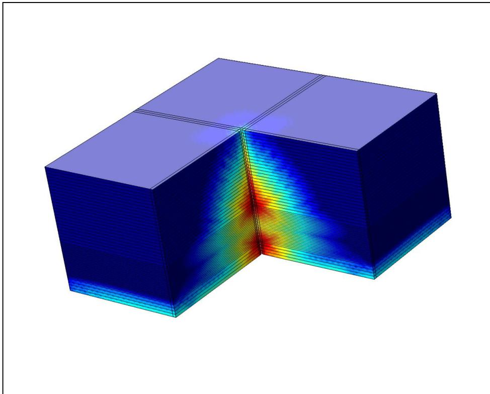
**Figure 5.** Example of 3D EM power field in the reservoir volume induced by the emitter in the center.
