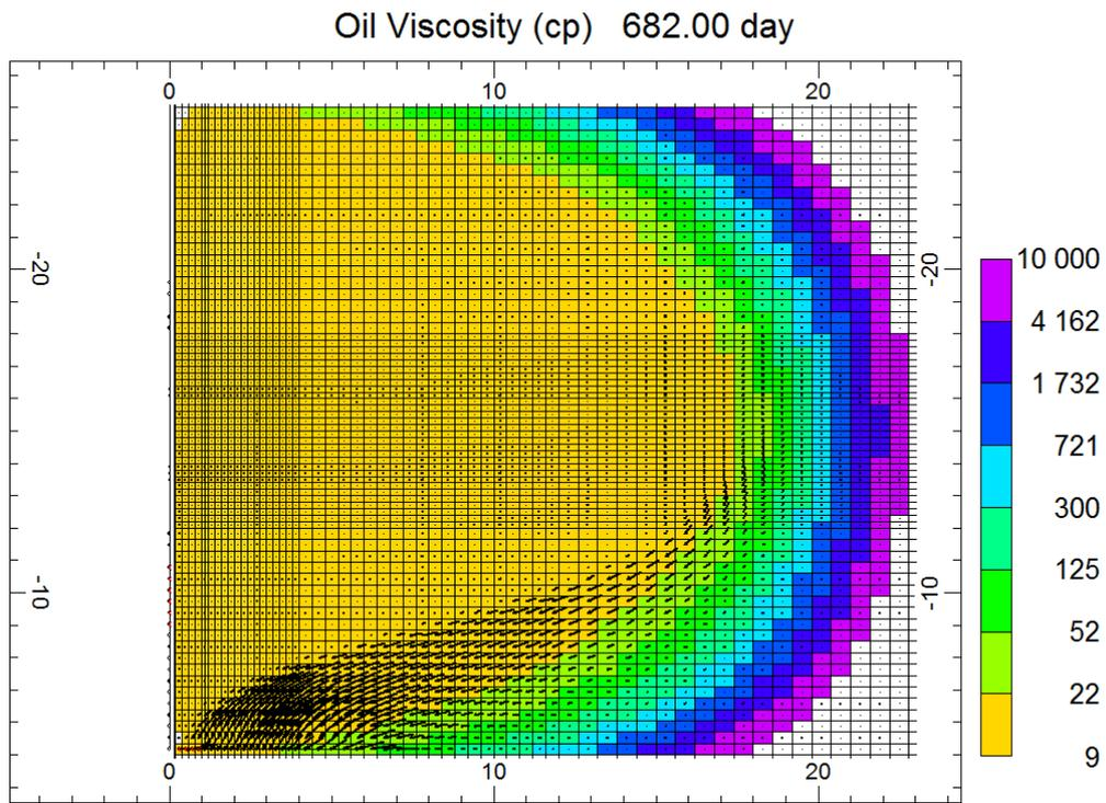
**Figure 4.** Oil viscosity field and flow lines towards production well; initial oil viscosity is  $10^6$  cP
