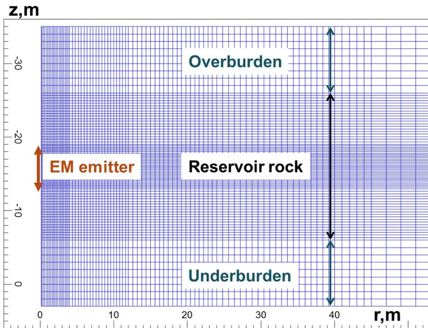
**Figure 1.** Geometry and the reservoir simulator grid.
