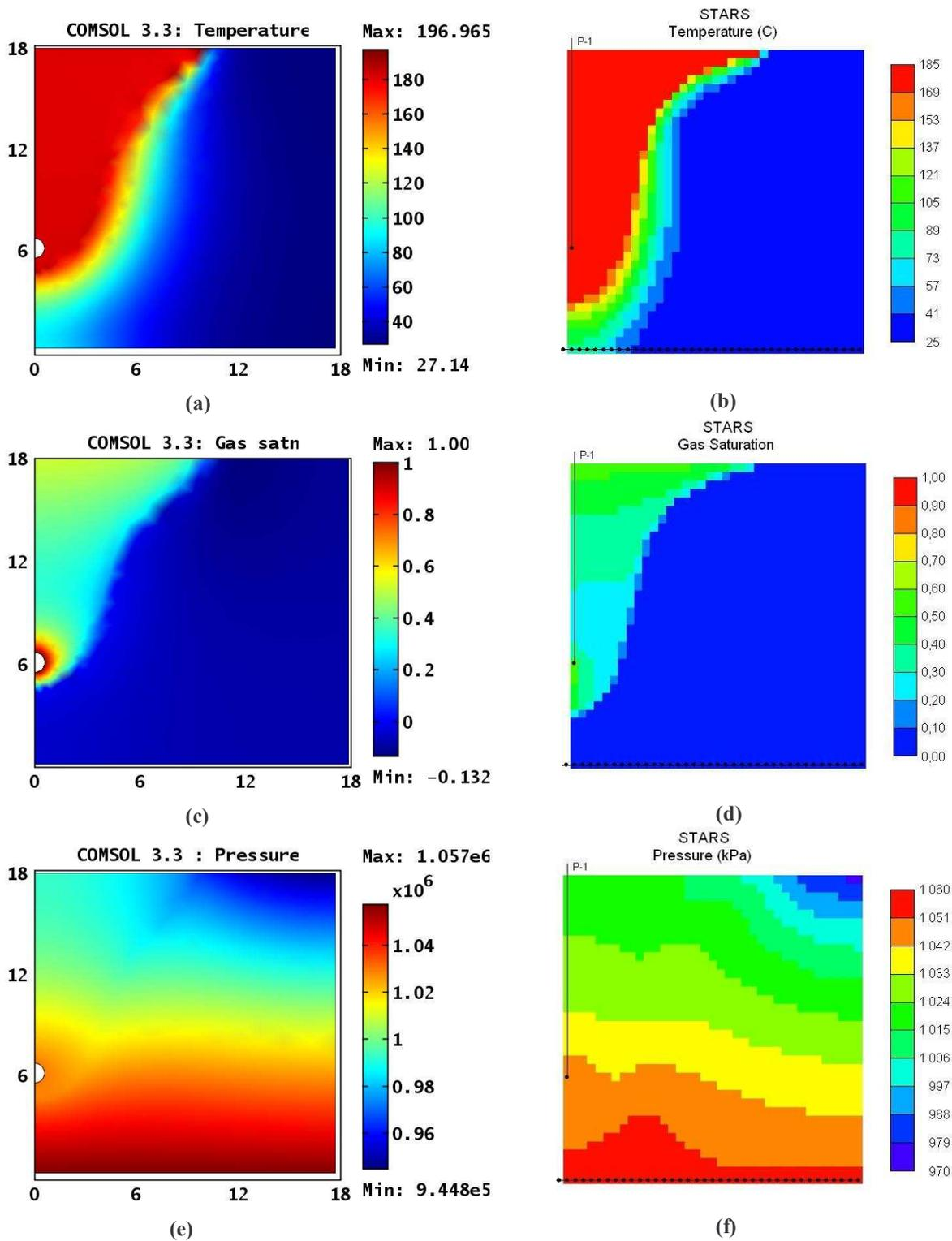
**Figure 2.** Comparison of COMSOL model to similar STARS model results: temperature fields (a,b), in C, gas saturation fields (c,d) and pressure fields (e,f), in Pa for COMSOL, (e), and in KPa for STARS, (f), after injection of steam amount equivalent to 4.08 m<sup>3</sup> of liquid water at reservoir conditions
