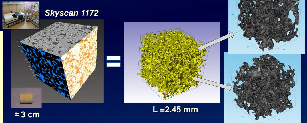
**Figure 1.** The *Bentheimer* rock sample (bottom left insert), raw reconstructed slice (left image: upper face), sample texture (right face), segmentation (left face); extracted pore volume (middle image) resulted from post processing in *ScanIP*; grid examples (COMSOL, right images).
