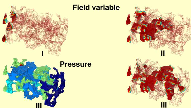
**Figure 2.** Drainage at three different PV injected (I to III),  $\text{NC} \approx 3 \cdot 10^{-7}$ , viscosity ratio 1, constant flowrate (BC2), no gravity,  $S_{\text{nwet}} \approx 0.51$  (III).
