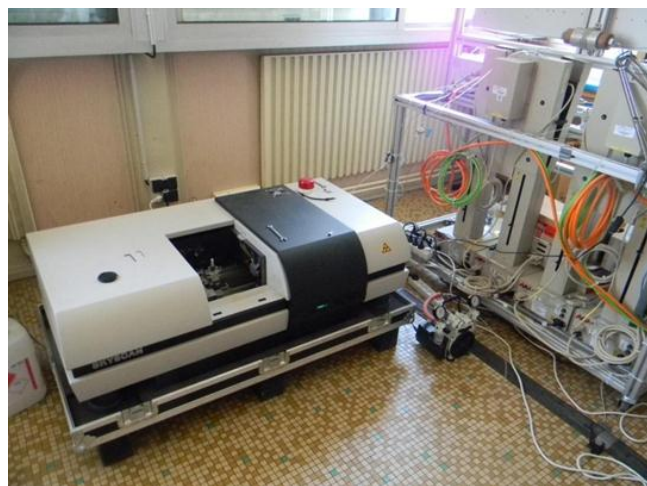
Figure 1 Laboratory setup with the Skyscan 1172 microtomograph and the Bentheimer sample inside.
