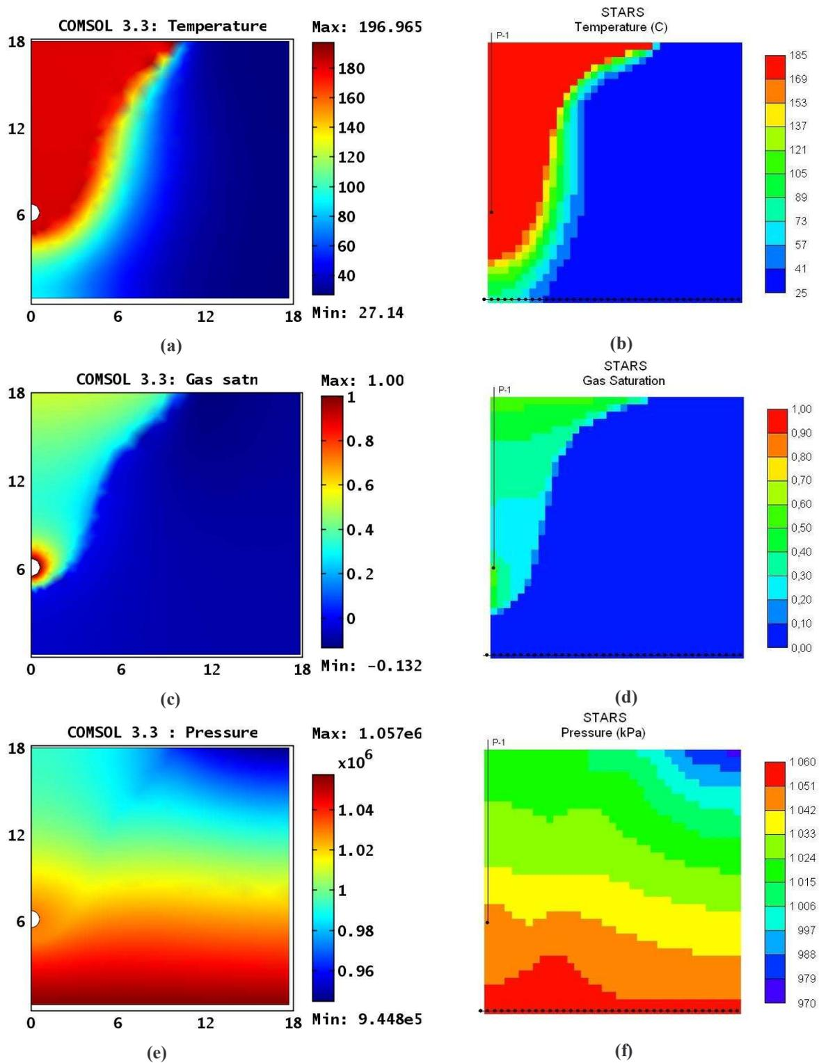
**Figure 2.** Comparison of COMSOL model to similar STARS model results: temperature fields (a,b), in C, gas saturation fields (c,d) and pressure fields (e,f), in Pa for COMSOL, (e), and in KPa for STARS, (f), after injection of steam amount equivalent to  $4.08 \text{ m}^3$  of liquid water at reservoir conditions
